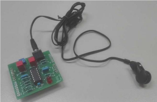
Figure 3: Heart rate monitor PCB based on photoplethysmography
